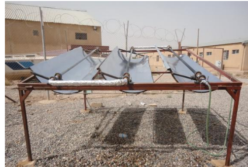
Figure 4a Structure system of solar concentrator trough.
