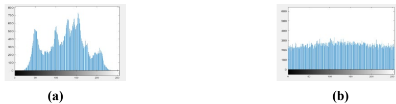
Fig.5: Plot of histograms (a) For test input 'Lena' (b) For chaotic map encrypted image
